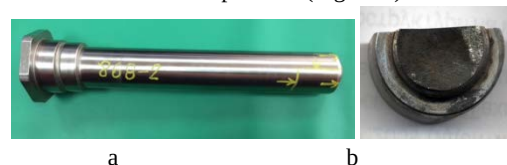
Figure 2 (a and b) fractured pin b broken surface of pin
